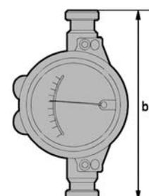
① Stainless steel 1.4435 - EHEDG tested - wetted surfaces Ra ≤ 0.8 / 0.6 µm
