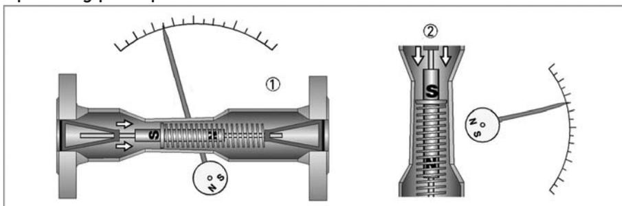
Figure 1-1: Operating principle H250H and H250U
