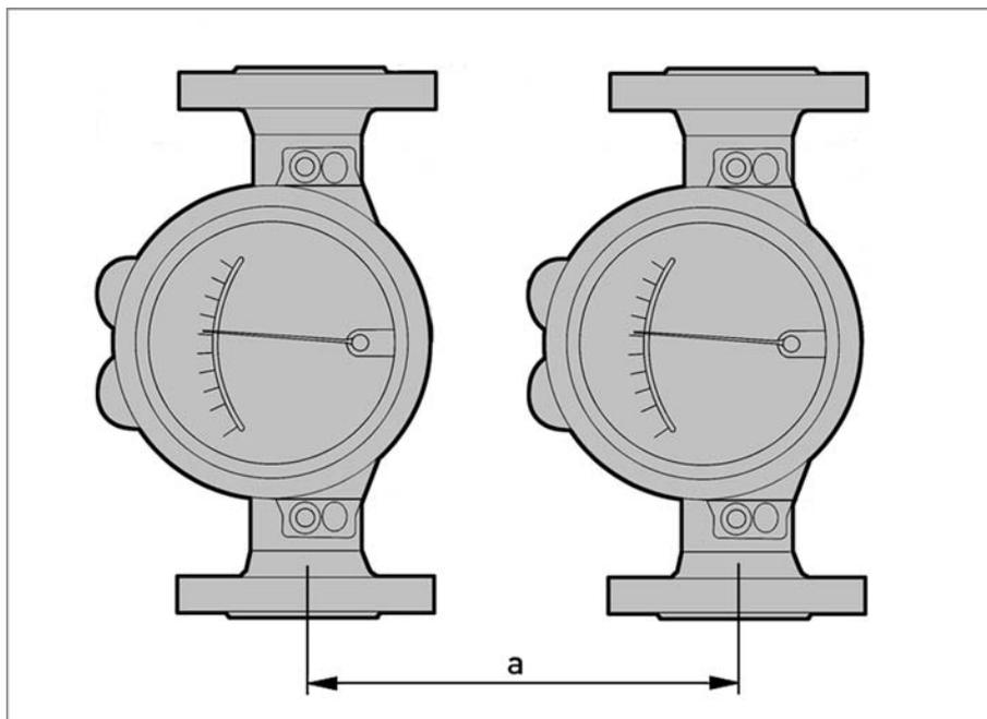
Take special note of the installation position for the H250H with horizontal flow direction:
