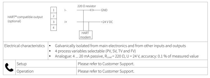
Table 18: Wiring HART® compatible output
