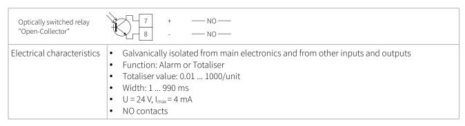
Table 15: Wiring digital open-collector output using expansion junction box
