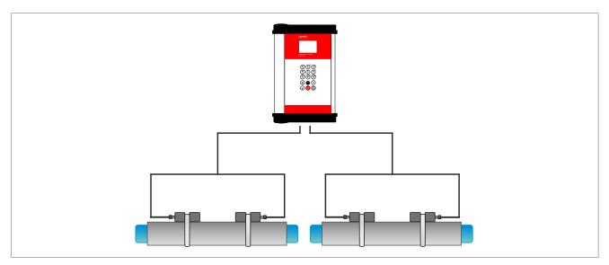
Picture 4: KATflow 230 in a 2-pipe 1-path configuration
