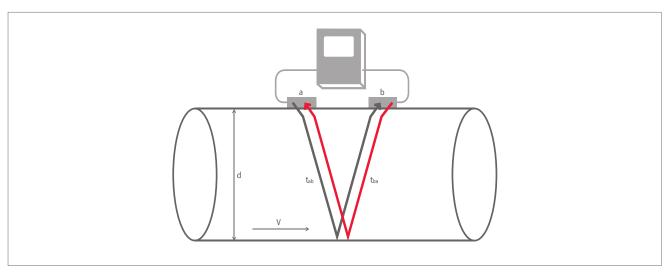
Picture 1: Clamp-on ultrasonic flowmeter configuration
