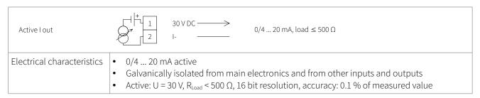
Table 13: Wiring analogue current output 0/4 ... 20 mA using expansion junction box
