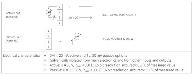
Table 19: Wiring analogue current output 0/4 ... 20 mA
