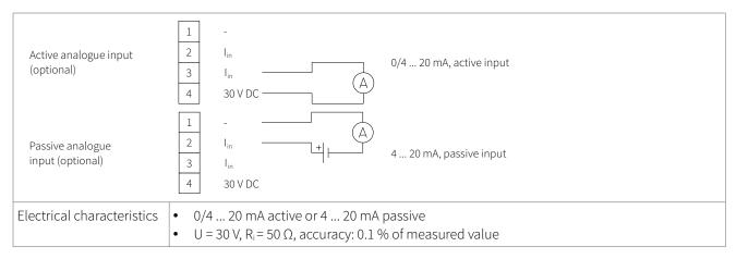
Table 25: Wiring analogue current input 0/4 ... 20 mA
