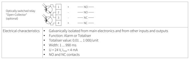
Table 22: Wiring digital open-collector output
