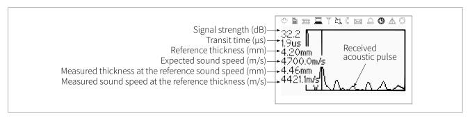
Picture 19: Wall Thickness Gauge (WTG) screen
