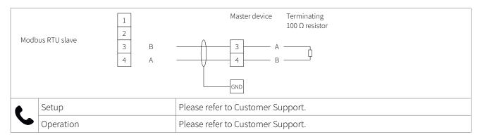
Table 17: Wiring Modbus RTU
