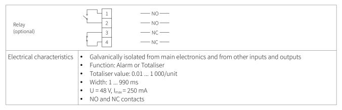
Table 23: Wiring digital relay output
