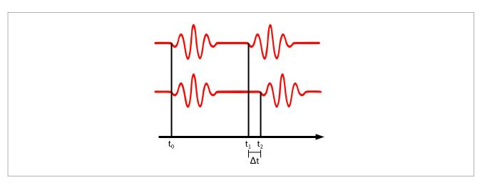
Picture 2: Transit-time measuring principle
