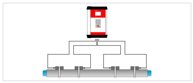
Picture 3: KATflow 230 in a 1-pipe 2-path configuration
