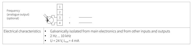
Table 21: Wiring analogue frequency output (passive)
