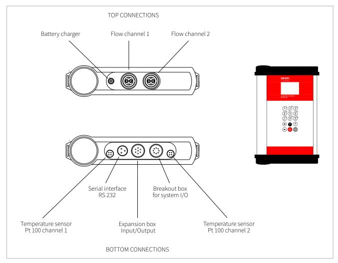
Picture 8: Electrical connection diagram KATflow 230
