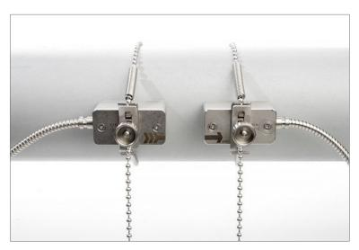
Picture 8: Correct positioning of the sensors
