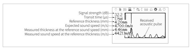
Picture 14: Wall Thickness Gauge (WTG) screen
