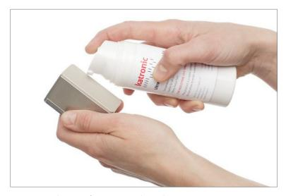
Picture 7: Application of acoustic coupling gel
