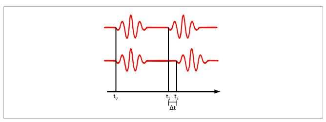
Picture 2: Transit-time measuring principle
