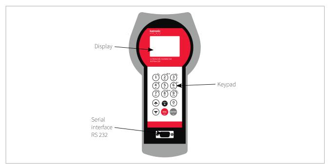
Picture 12: Keypad and display KATflow 200
