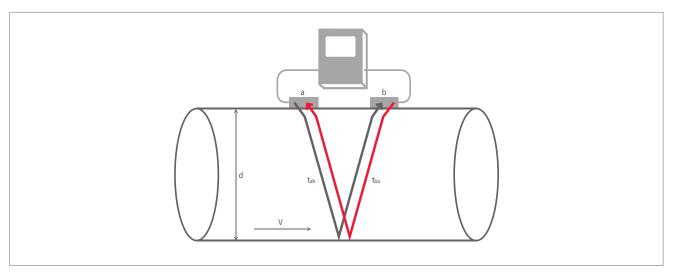
Picture 1: Clamp-on ultrasonic flowmeter configuration
