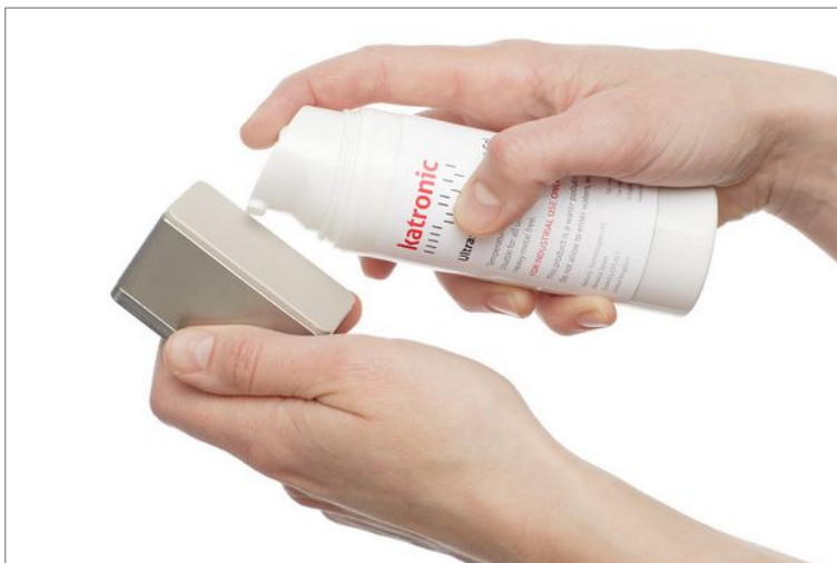
Picture 7: Application of acoustic coupling gel
