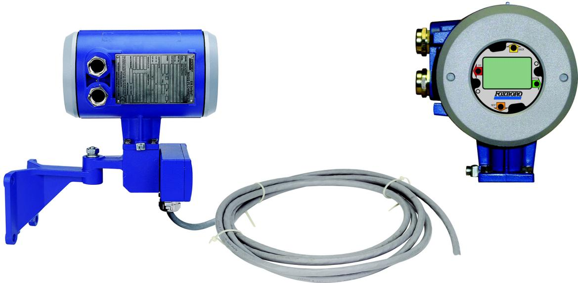
*The Foxboro® brand Model CFT50 Digital Coriolis Mass Flow Transmitter combines with a Model CFS10 or CFS20 Mass Flowtube to form an I/A Series Mass Flow and Density Meter. Use of digital signal processing (DSP) techniques provides enhanced flowmeter performance, and adds new features over previous transmitter versions. The CFT50 uses HART or Modbus protocol for remote communications.*
