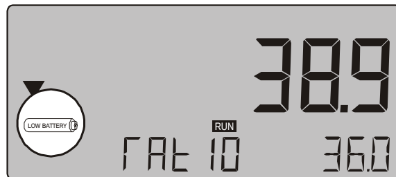
Fig. 5: Example of low-battery alarm.
