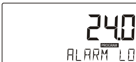
Fig. 4: Example of display information during programming minimum flowrate alarm.
