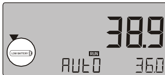
Fig. 4: Example of low-battery alarm.
