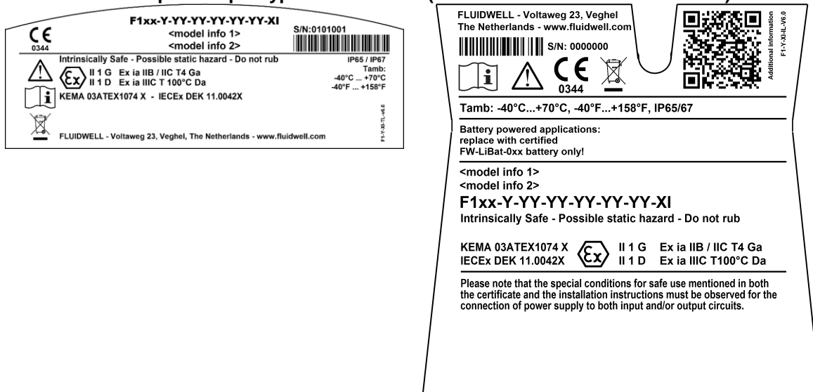
Fig. 26: Label information - Intrinsic safe application (typical)
