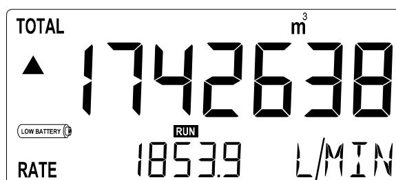
Fig. 5: Example of low-battery alarm.
