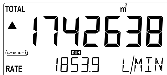
Fig. 4: Example of low-battery alarm.
