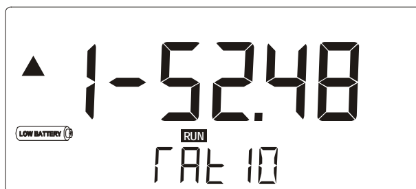
Fig. 5: Example of low-battery alarm.
