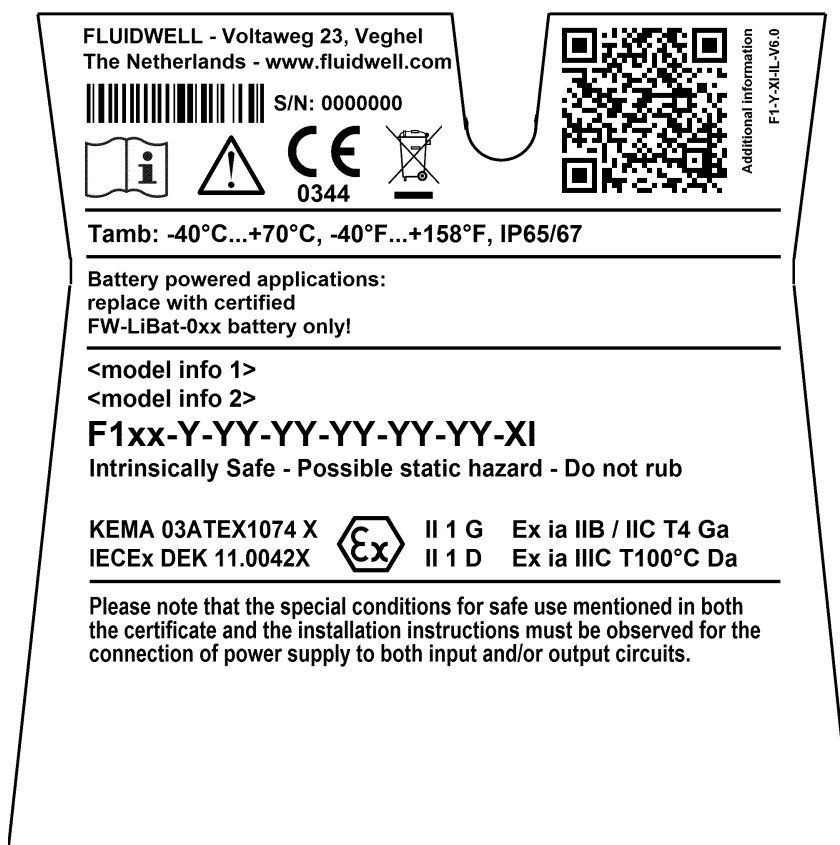
Fig. 27: Label information - Intrinsic safe application (typical)
