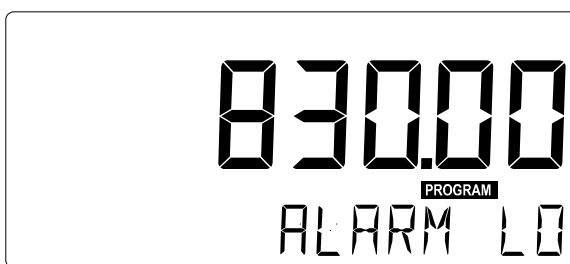
Fig. 4: Example of display information during programming minimum flowrate.
