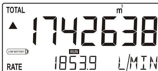
Fig. 5: Example of low-battery alarm.
