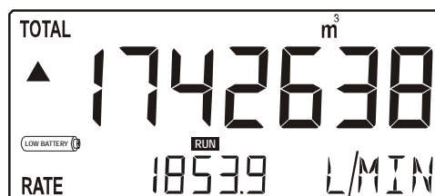
Fig. 4: Example of low-battery alarm.
