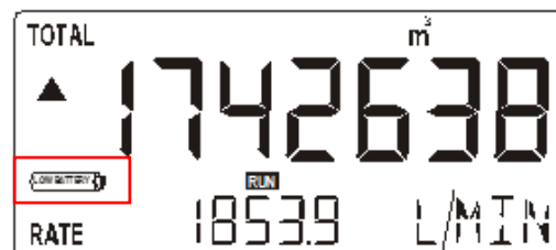
Fig. 4: Low-battery alarm (typical)
