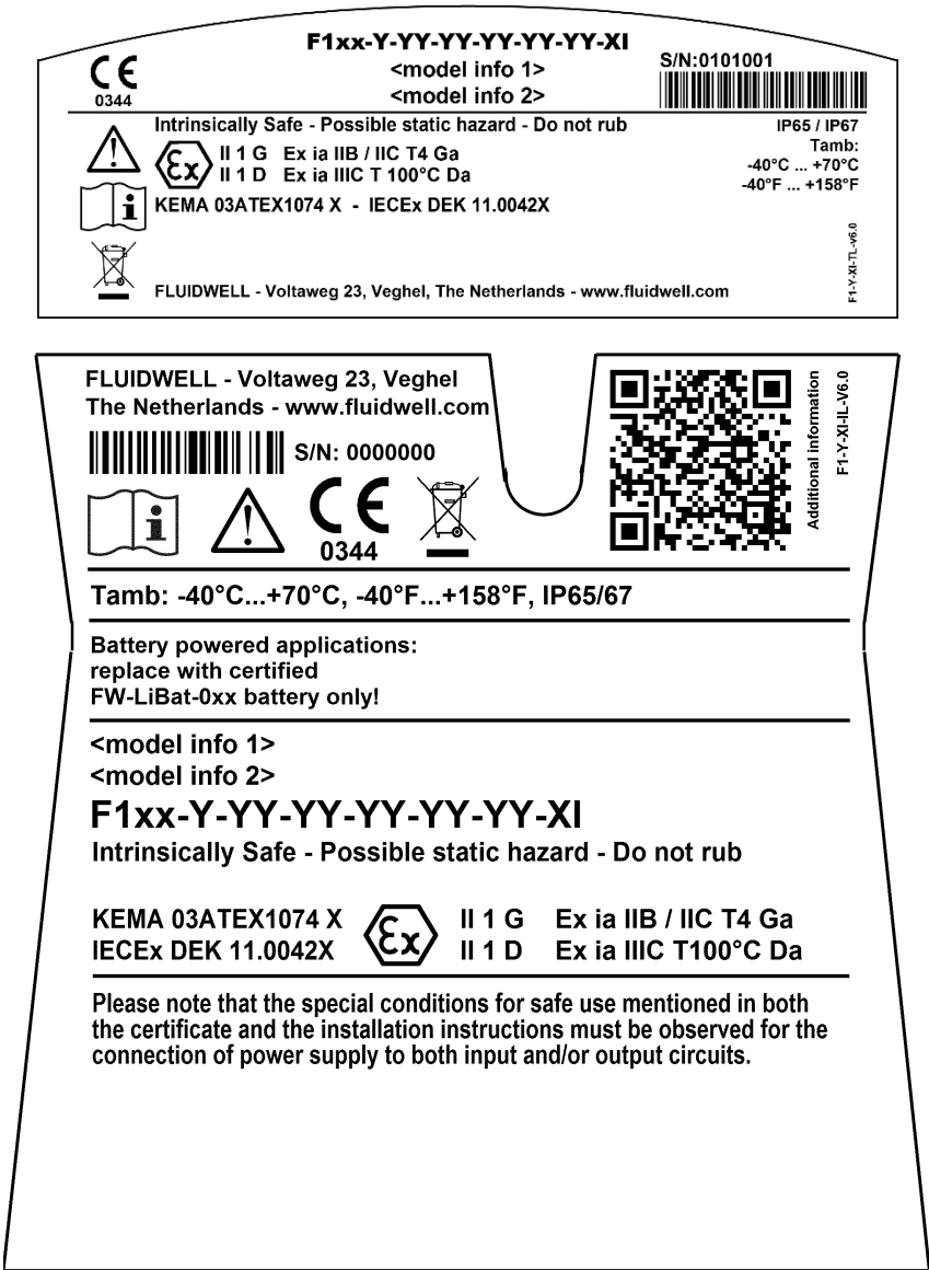
Fig. 21: Label information - Intrinsically safe application (typical)
