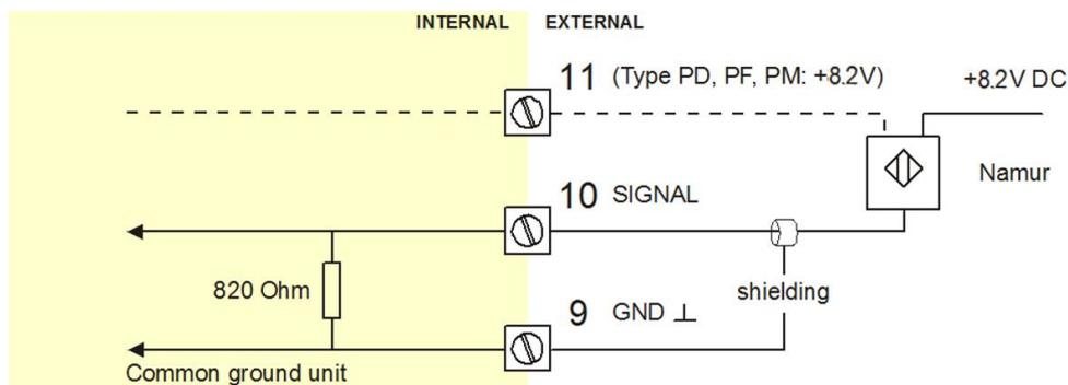
**Fig. 16: Terminal connections - NAMUR signal input (typical)**
