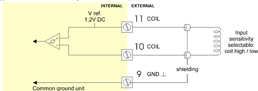
**Fig. 11: Terminal connections - Coil signal input (typical)**
