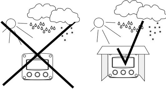
Take the relevant IP classification of the enclosure into account (see identification plate). Even an enclosure rated for IP67 / TYPE 4(X) should NEVER be exposed to strongly varying (weather) conditions.
