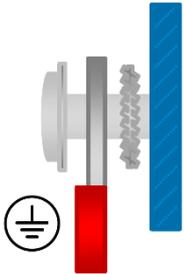
The PE connection in the metal back panel is made with a serrated washer, a terminal, a washer and a screw.
