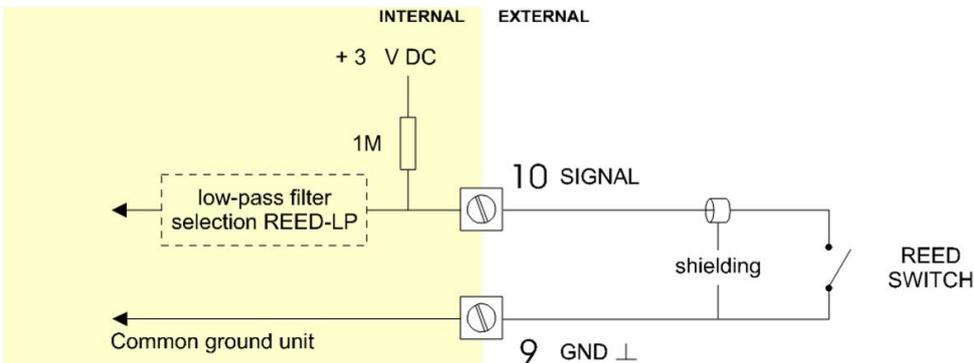
**Fig. 15: Terminal connections - Reed-switch signal input (typical)**
