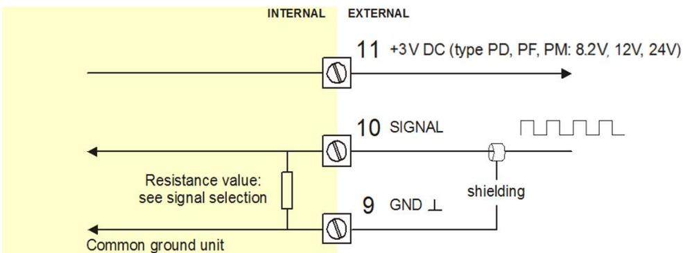
**Fig. 14: Terminal connections - Active signal input (typical)**
