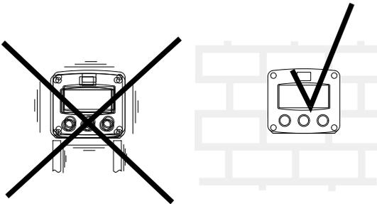
Mount the F111-P onto a solid structure to avoid vibrations.
