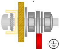
The PE connection to the metal cover is made with the serrated washers and the mounting screws.
