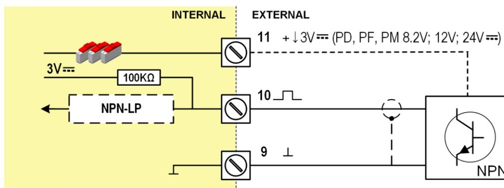
**Fig. 12: Terminal connections - NPN signal input (typical)**
