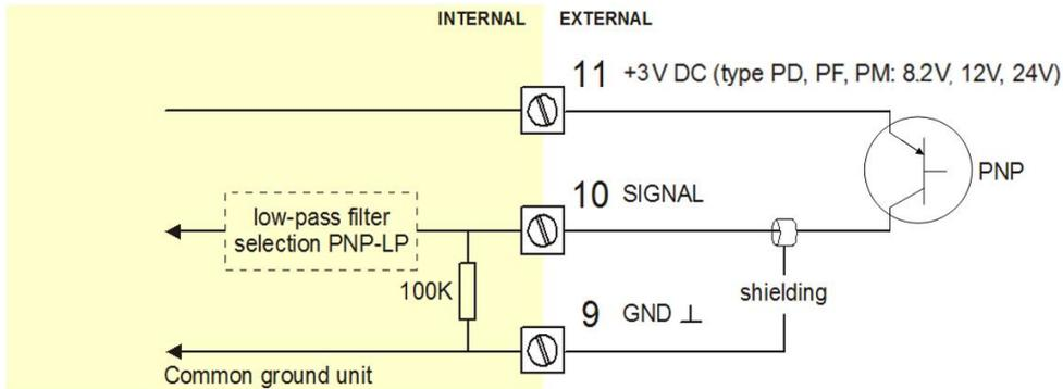
**Fig. 13: Terminal connections - PNP signal input (typical)**
