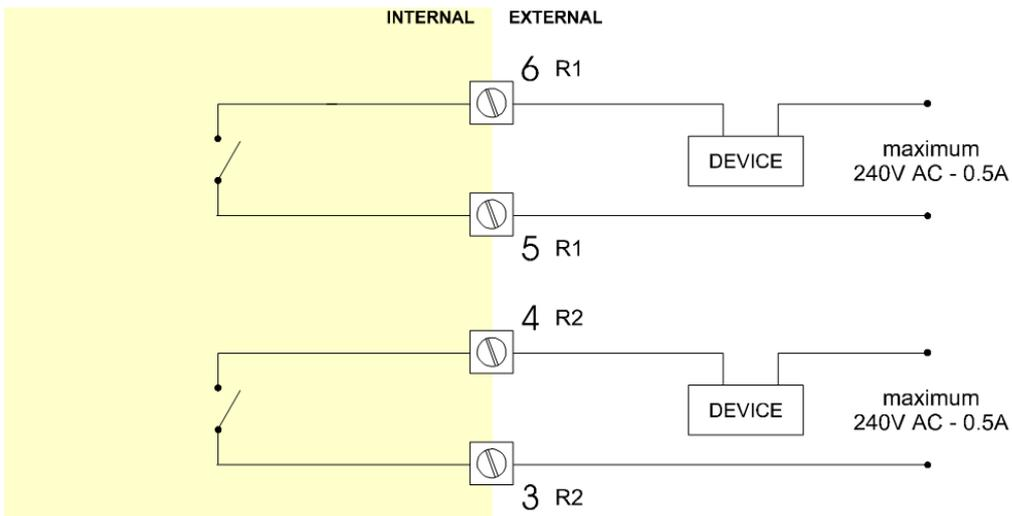
**Fig. 9: Terminal connections - Mechanical relay output (typical)**
