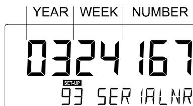
Fig. 17: Example serial number (typical)
