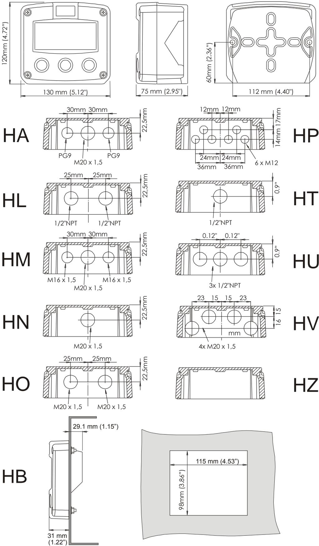
Fig. 4: Aluminum enclosures - Dimensions
