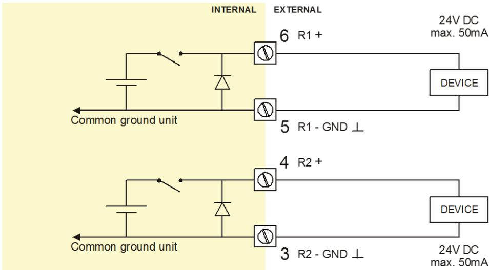
**Fig. 8: Terminal connections - Active output (typical)**
