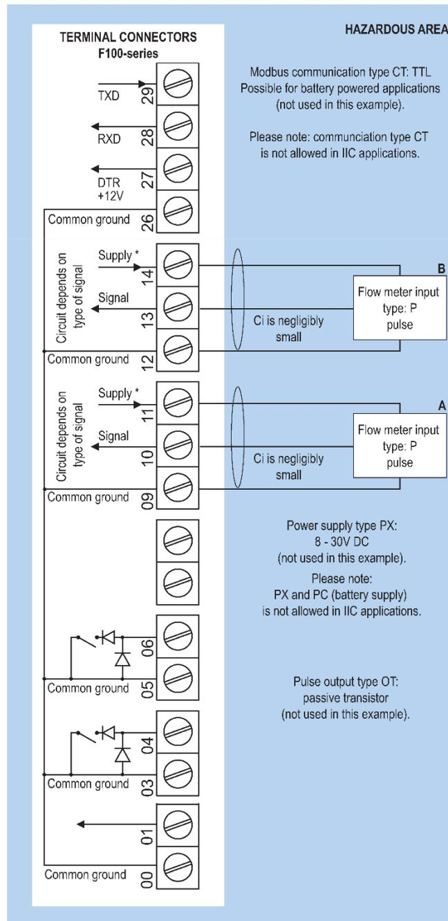
Fig. 21: F111-P-(AP)-(CT)-(OT)-PC-XI - Battery powered - IIB/IIC – IIIC
