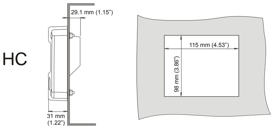
Fig. 5: GRP enclosures - Dimensions
