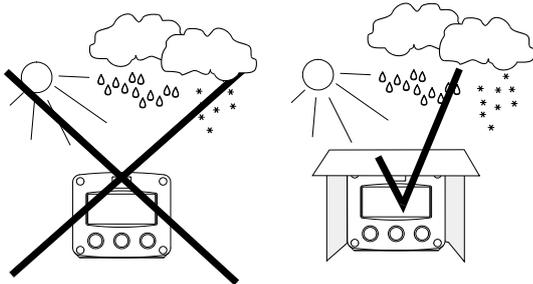
Take the relevant IP classification of the enclosure into account (see identification plate). Even an enclosure rated for IP67 / TYPE 4(X) should NEVER be exposed to strongly varying (weather) conditions.
