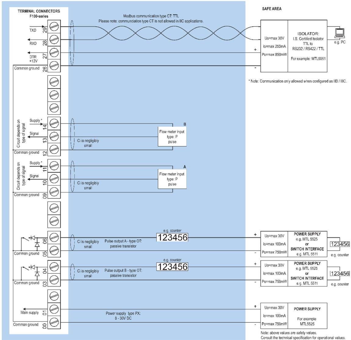
\* Note sensor supply voltage: 1.2V DC for coil sensors or 3.2V DC for other pulse sensors.
