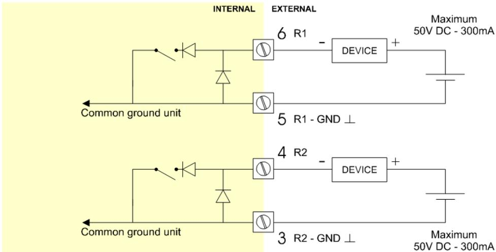
**Fig. 10: Terminal connections - Passive transistor output (typical)**
