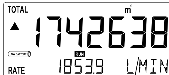
Fig. 4: Example of low-battery alarm
