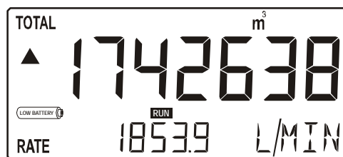
Fig. 4: Example of low-battery alarm
