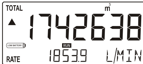
Fig. 4: Example of low-battery alarm.
