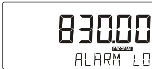
Fig. 5: Example of display information during programming minimum flowrate.
