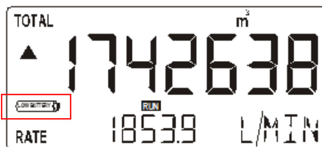
Fig. 4: Example of low-battery alarm.
