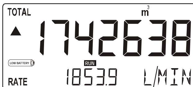
Fig. 4: Example of low-battery alarm.
