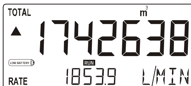
Fig. 4: Example of low-battery alarm.
