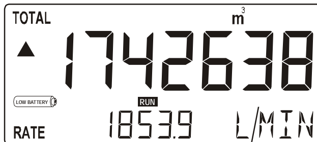
Fig. 5: Example of low-battery alarm.
