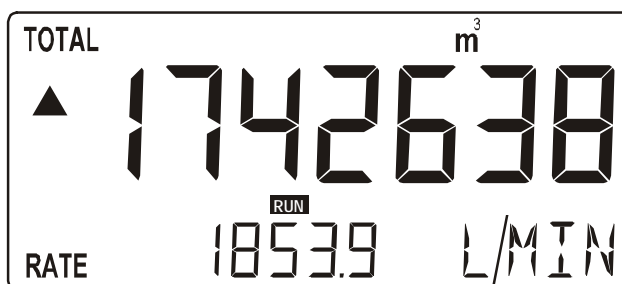
Fig. 3: Example of display information during process.
