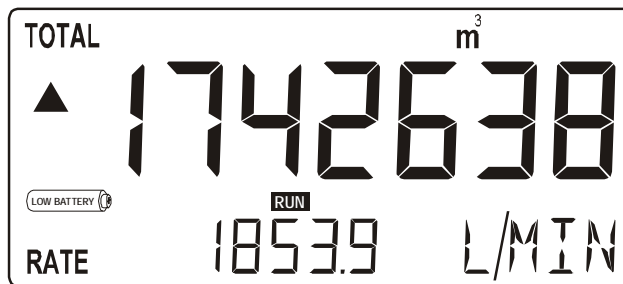
Fig. 5: Example of low-battery alarm.
