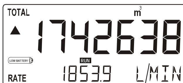
Fig. 4: Example of low-battery alarm.
