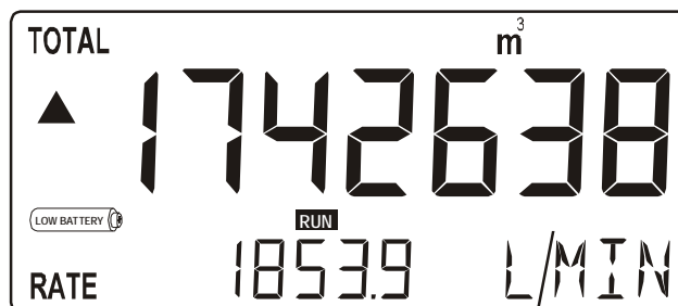
Fig. 4: Example of low-battery alarm.
