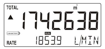
*Fig. 4: Example of low-battery alarm.* HF012AEN\_v0403\_03 Atex\_IECEx\_CSA\_FM
