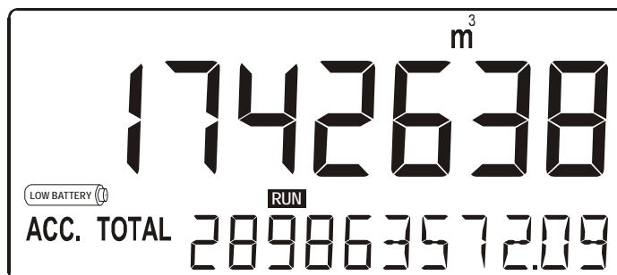
Fig. 4: Example of low-battery alarm.
