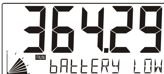
Fig. 4: Example of low-battery alarm.
