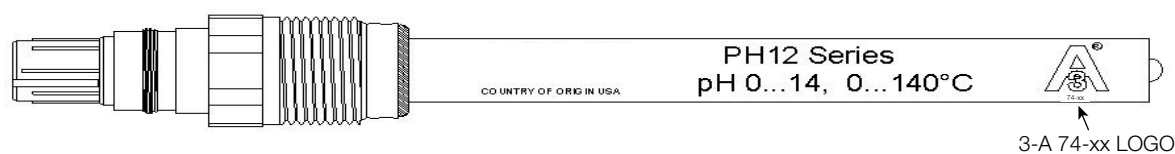
Figure 3. 3-A 74-xx Compliant Sensor
