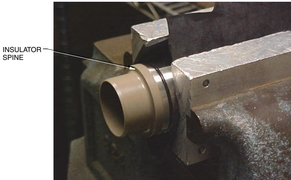
7. Lubricate the new O-rings with the silicone grease supplied in the O-ring kit.
