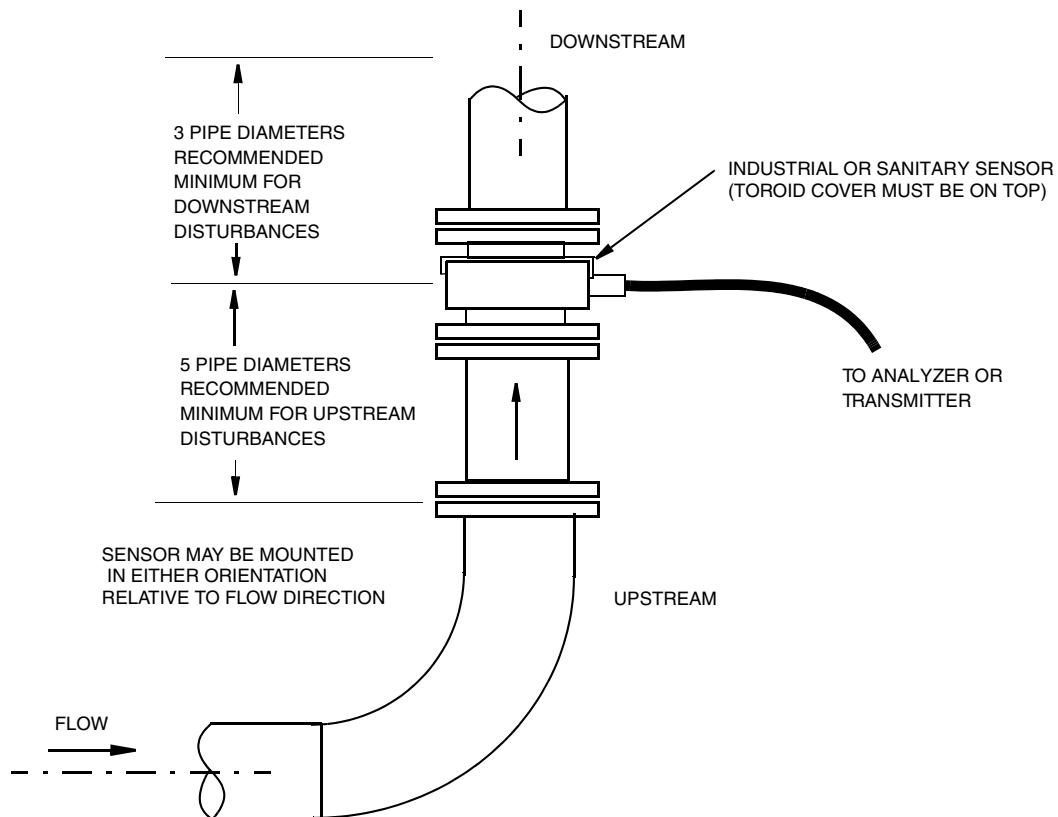
*Figure 11. Horizontal Mounting of Sensor*
