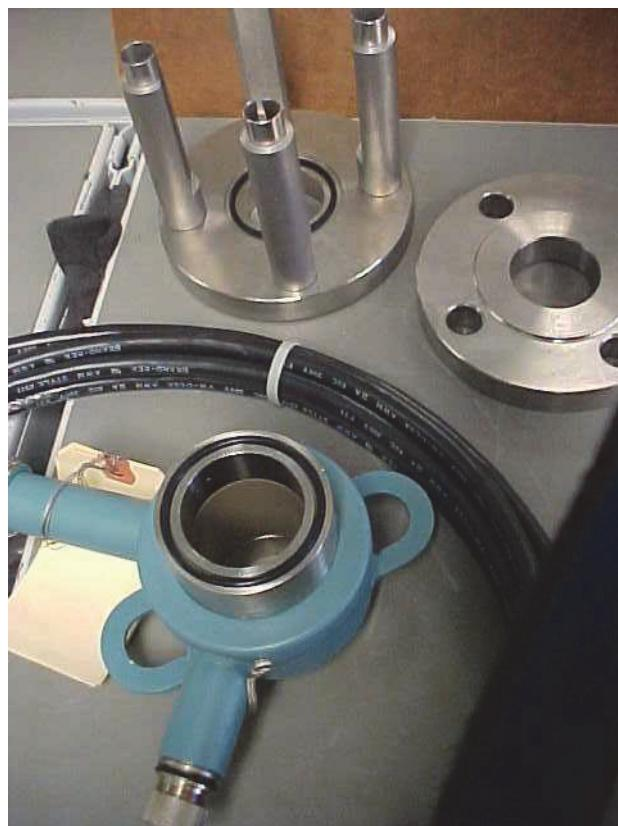
4. Carefully remove one toroid sleeve from the toroid assembly.
