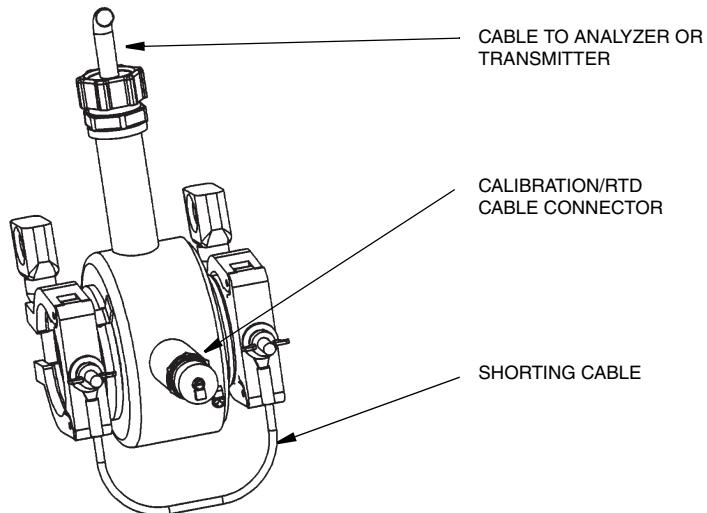
*Figure 2. 871FT Conductivity Sensor – Industrial Version (Flanged)*
