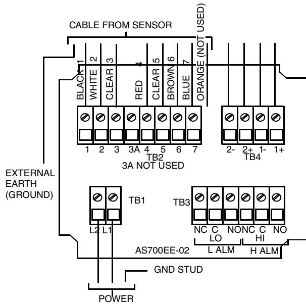
The plastic NEMA 1 Analyzer should be used only with the Teflon-jacketed cable, since provision is not otherwise made for metal conduit connection to this instrument. The orange lead No. 8 from the sensor is not used and the ground lead with the eye terminal is connected to the green wire power ground terminal on the back of the analyzer.
