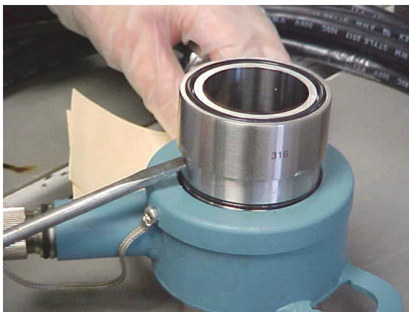
5. After removal of one toroid sleeve, the other sleeve and the insulator (bore piece) can easily be removed from the toroid assembly. You can now see the inner and outer toroid sleeve O-rings.
