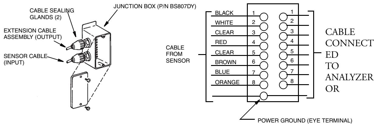
**Figure 20. Junction Box Wiring with 8-Conductor PVC-Jacketed Cable**
