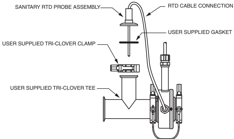
*Figure 7. Temperature Compensation Assembly With Industrial Sensors*
