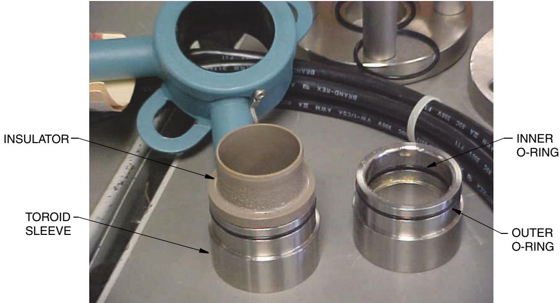
6. Grab the toroid sleeve, either by hand or by some mechanical means (as shown) and carefully remove the insulator using a twisting motion. Even though the toroid sleeve is well lubricated with silicone grease, sometimes it is necessary to use a strap wrench on the spine of the insulator to start the rotation of the insulator in the sleeve.
