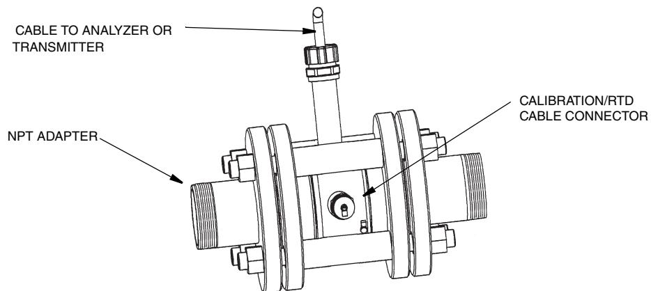
*Figure 3. 871FT Conductivity Sensor – Industrial Version (NPT)*
