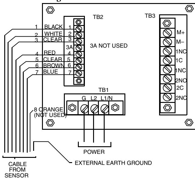
*Figure 16. Sensor Wiring to Metal 873EC and 873AEC NEMA 4X Analyzer*
