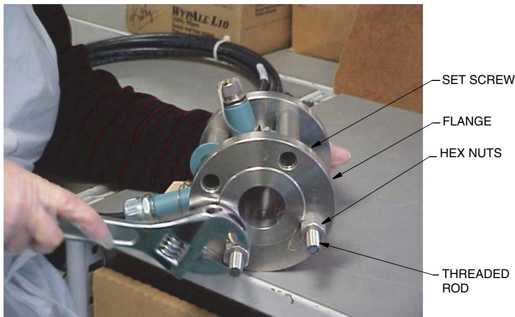
2. Loosen the set screws on the edge of one flange so the flange can be removed from the spacers.
