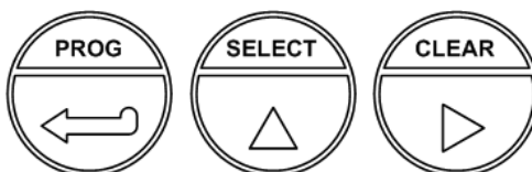
Fig. 2: Control panel, optical keys.
