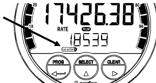
Fig. 7: Example of low-battery alarm.
