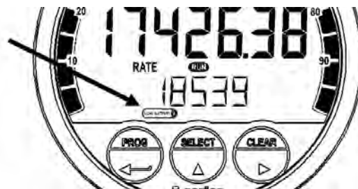
Fig. 7: Example of low-battery alarm.
