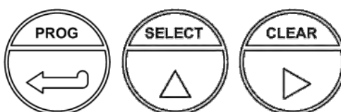
Fig. 2: Control panel, optical keys.
