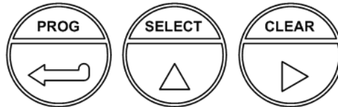
Fig. 2: Control panel, optical keys.
