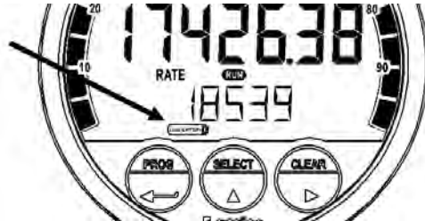
Fig. 7: Example of low-battery alarm.
