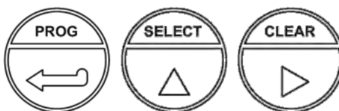
Fig. 2: Control panel, optical keys.
