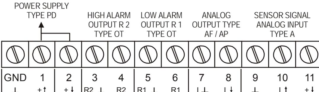
Fig. 13: Overview terminal connectors XI - Intrinsically Safe applications.
