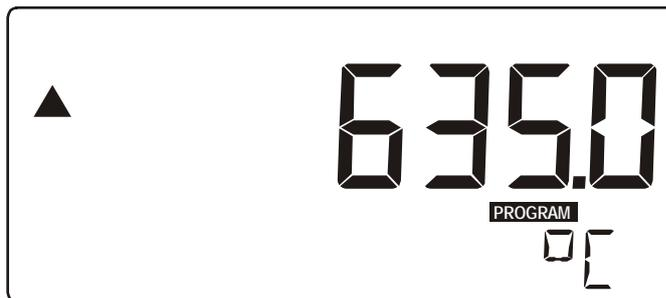
Fig. 4: Example display information during increasing / decreasing preset value.
