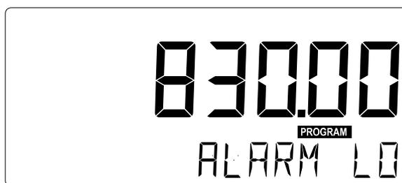
Fig. 4: Example of display information during programming low alarm value.
