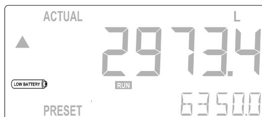
Fig. 5: Example of low-battery alarm.
