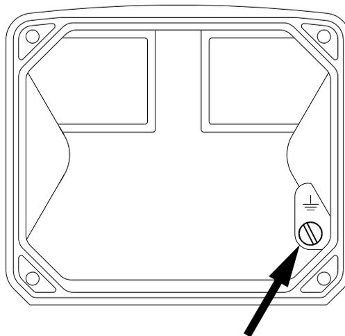
*Fig. 8: Grounding aluminum enclosure with type PM 115-230V AC.*
