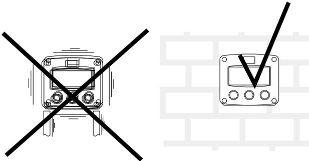
Mount the F197-A on a solid structure to avoid vibrations.
