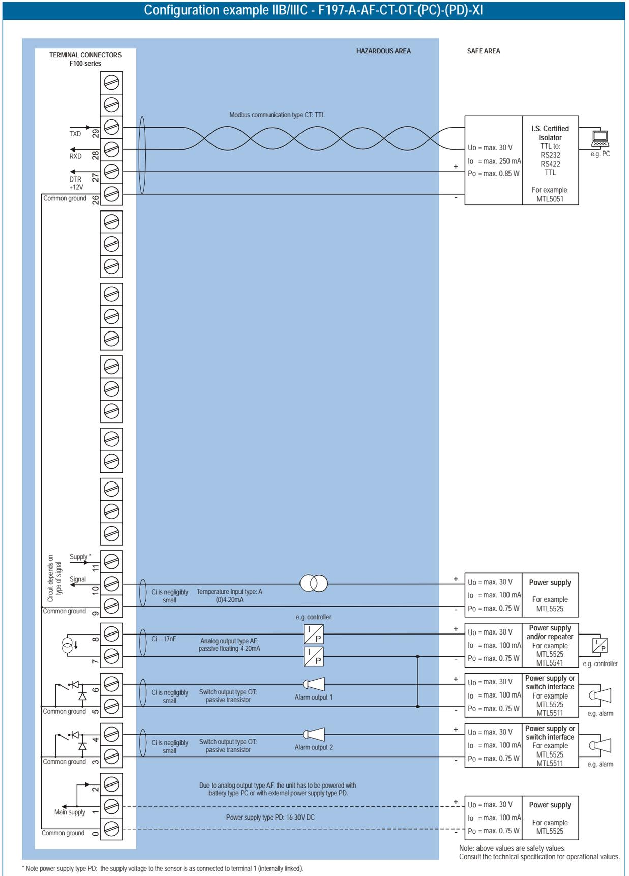
Fig. 14: Configuration example 1 Intrinsically Safe.
