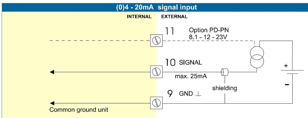
**Terminal 09-10: Type A-PL – sensor input / power supply:**
