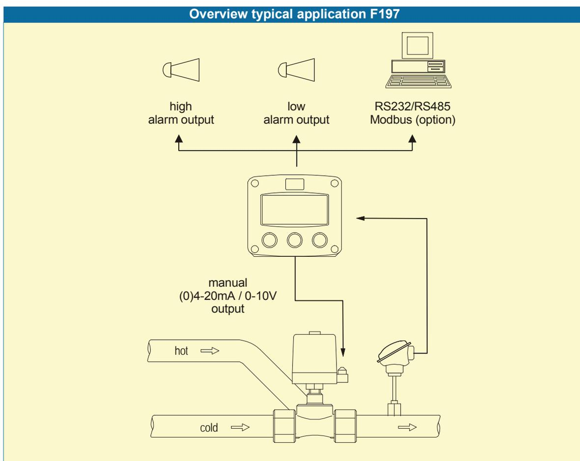
Fig. 1: Typical application for the F197-A.
