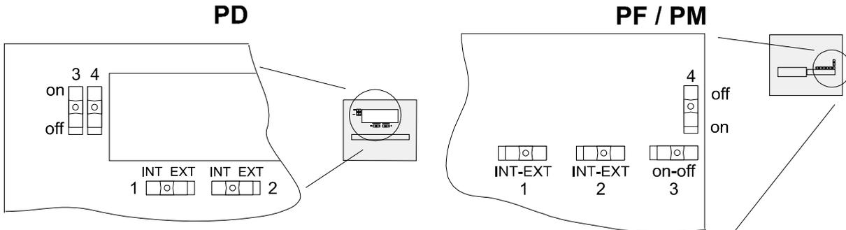
Fig. 9: switch position voltage selection (type PD / PF / PM).
