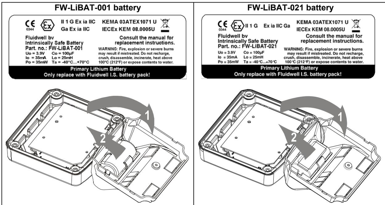
1. To replace the battery, open the unit to gain access to the back inside cover of the unit
