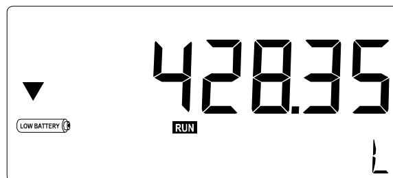
Fig. 5: Example of low-battery alarm.
