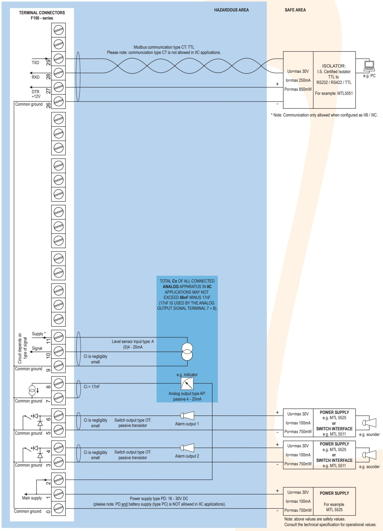
\* Note power supply type PD: the supply voltage to the analog sensor is as connected to terminal 1 (internally linked).
