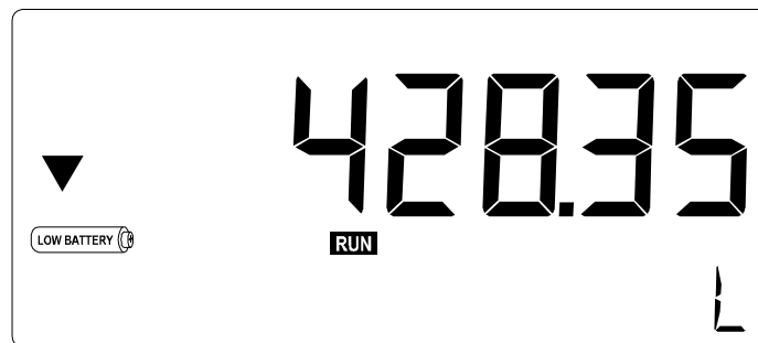
Fig. 5: Example of low-battery alarm.
