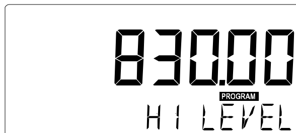
Fig. 4: Example display information during programming maximum level.
