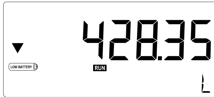
Fig. 5: Example of low-battery alarm.
