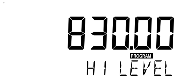
Fig. 4: Example display information during programming maximum level.
