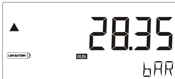
Fig. 5: Example of low-battery alarm.
