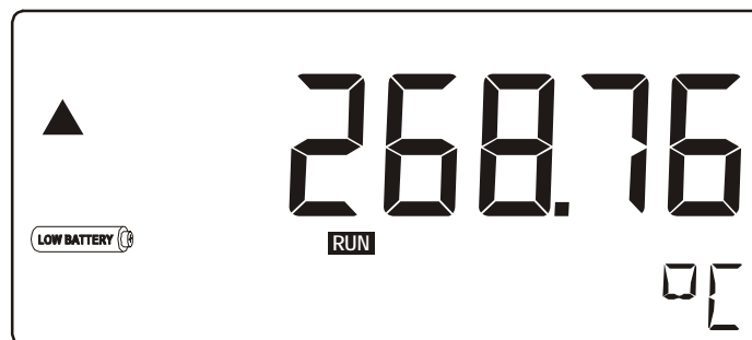
Fig. 5: Example of low-battery alarm.
