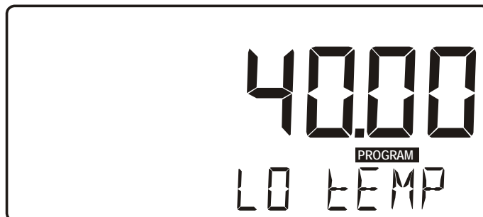
Fig. 4: Example display information during programming maximum temperature.
