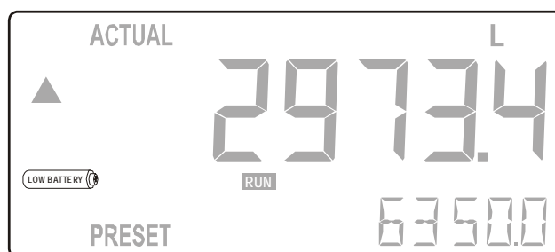
Fig. 6: Example of low-battery alarm.
