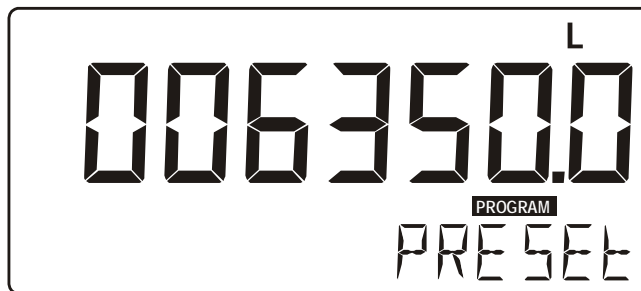
Fig. 3: Example display information during programming preset value.
