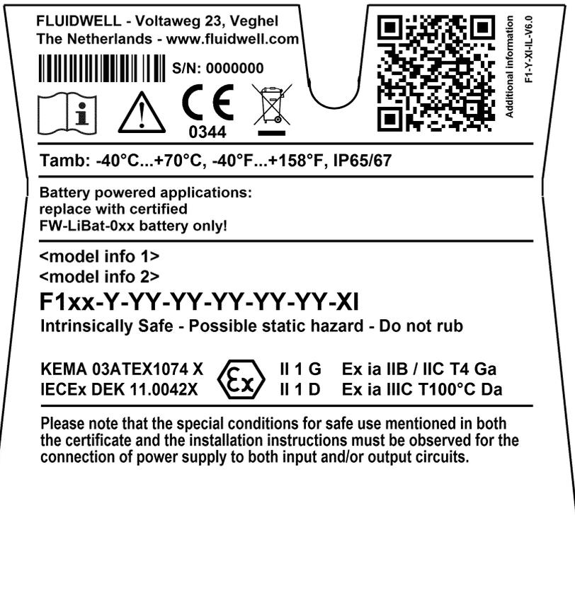
Fig. 25: Label information - Intrinsically safe application (typical)
