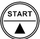
This key is used to START the batch process. The START/▲ key is also used to increase a value after the PROG/ENTER key has been pressed (read chapter 3). For setup of the printer, the START/▲ key is used to increase the value of the selected digit.
