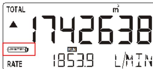
**Fig. 7: Example of low-battery alarm**
