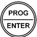
This key is used to program and save new values or settings. The PROG/ENTER key is also used to gain access to the setup menu (read chapter 3). For the setup of the printer, the PROG/ENTER key opens/closes the text edit mode.
