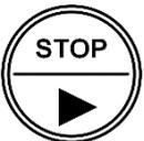
This key is used to pause or stop the batch process. When the batch process is stopped, it cannot be continued. The STOP/▶ key is also used to select the total, accumulated total and batch counter as well as a menu option to print a batch receipt. The STOP/▶ key is also used to select a digit or an option after the PROG/ENTER key has been pressed (read chapter 3).
