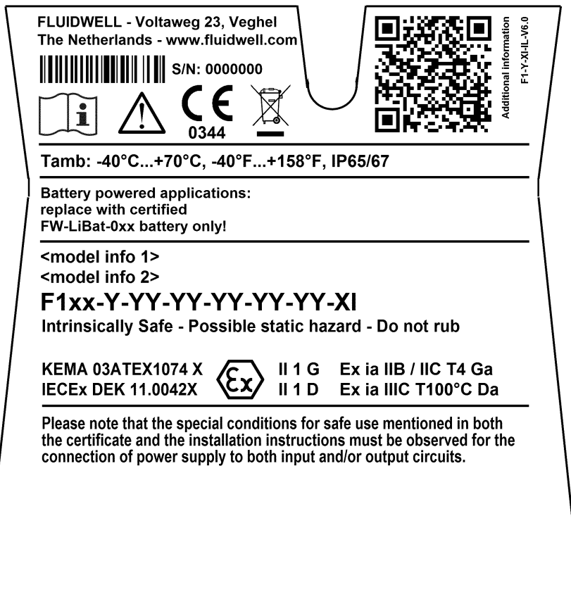
Fig. 29: Label information - Intrinsically safe application (typical)
