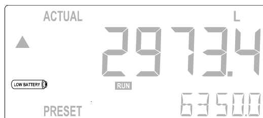
Fig. 6: Example of low-battery alarm.
