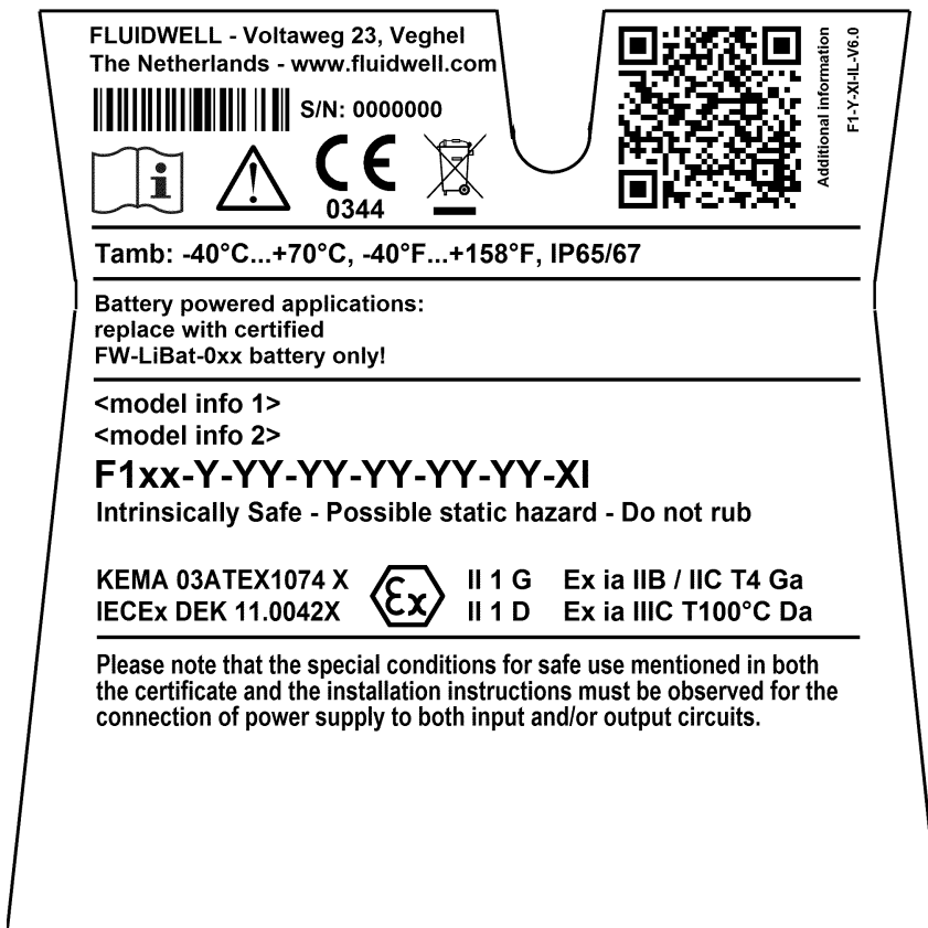
Fig. 24: Label information - Intrinsically safe application (typical)
