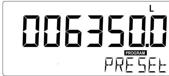
Fig. 3: Example display information during programming preset value.
